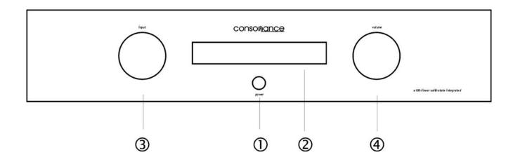
The amplifier is switched on with the button ① in the middle of the front panel. A flashing " -- -- blue light in the display ② indicates that power is switched on. By pushing the same button one more time the power is switched off.
